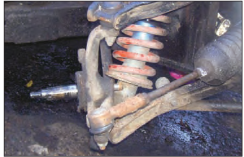
Bare Shaft and steering arm locknut undone, ready to take hub
